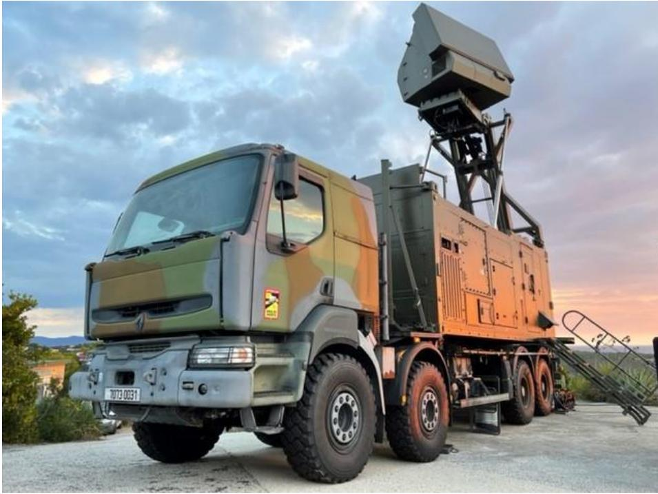
Ground Master radars 200 and 400 are multi-mission 3D air surveillance radars, tactical medium-range (~200 km) with the GM200 and fixed or mobile long-range (~400 km) with the GM400.
